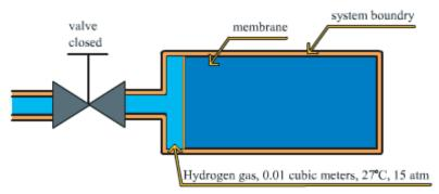
Basis:  $0.01 \text{ m}^3$  of  $H_2$  at  $27^{\circ}$ C, 15 atm.
