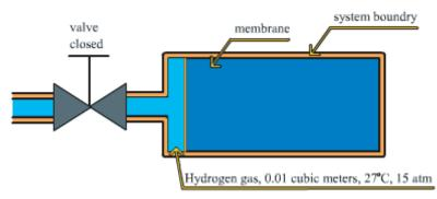
Basis: 0.01  $\text{m}^3$  of H<sub>2</sub> at 27°C, 15 atm.
