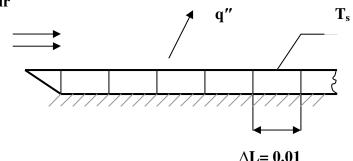
**Take**: Air (T<sub>f</sub> = 535 K, 1 atm):  $v = 43.54 \cdot 10^{-6} \text{ m}^2/\text{s}$ , K = 0.0429 W/m·K, Pr = 0.683. (17 marks)
