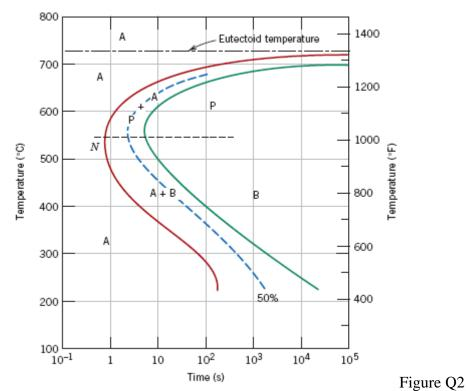
Figure Q2 is an isothermal transformation diagram for a steel of eutectoid composition. Using it as a reference, describe the following heat treatment processes.
